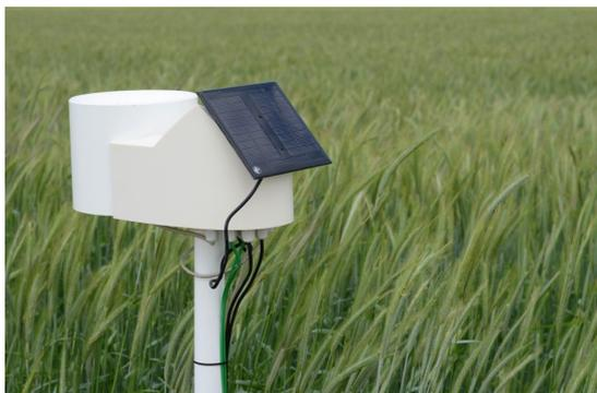
1. M-Metos Soil Base - DTU with rain gauge
