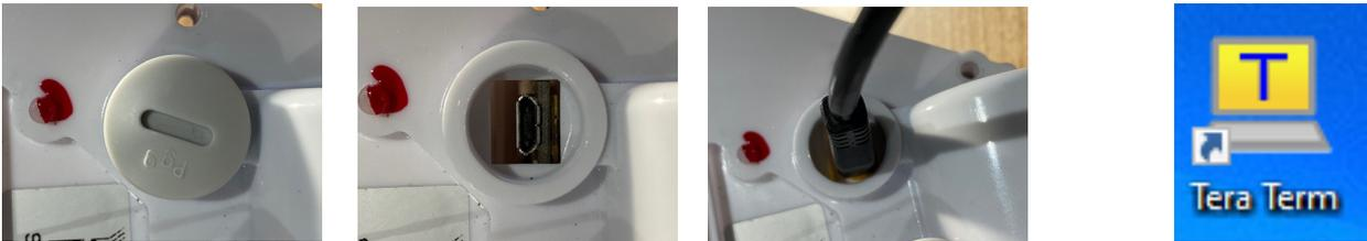
Remove the Comms cover and connect the comms cable as shown above. Not all METOS units will have port access such as is pictured above, LoRATH and LoRain units do. The probe DTU units do not but may have a flying lead as an access point.
