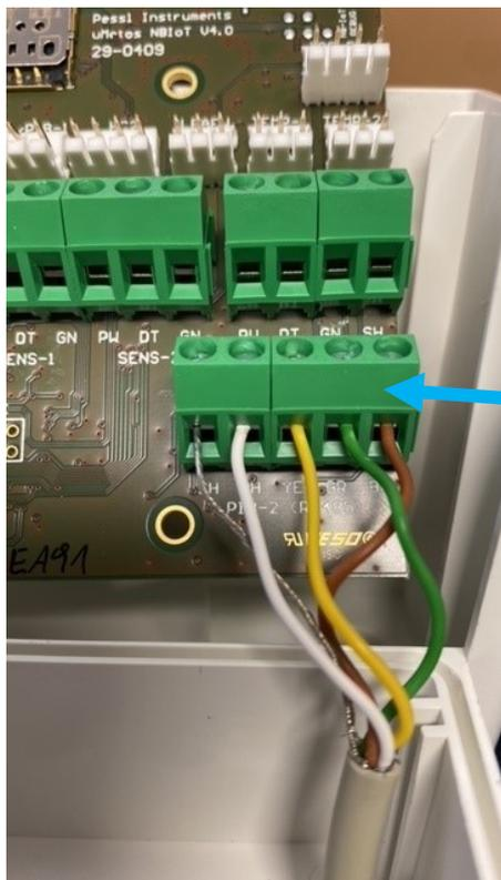
pH / EC interface wiring on to 0390 / 0310 board
