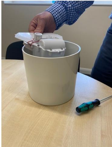
Once the first peg is released remove tipper unit from the rain gauge body
