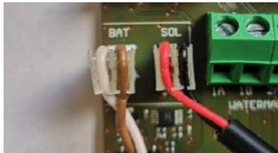
Picture 13 – Left: Battery cable, right: solar panel cable
