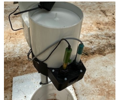
Rain Gauge with added EC / pH sensor well
