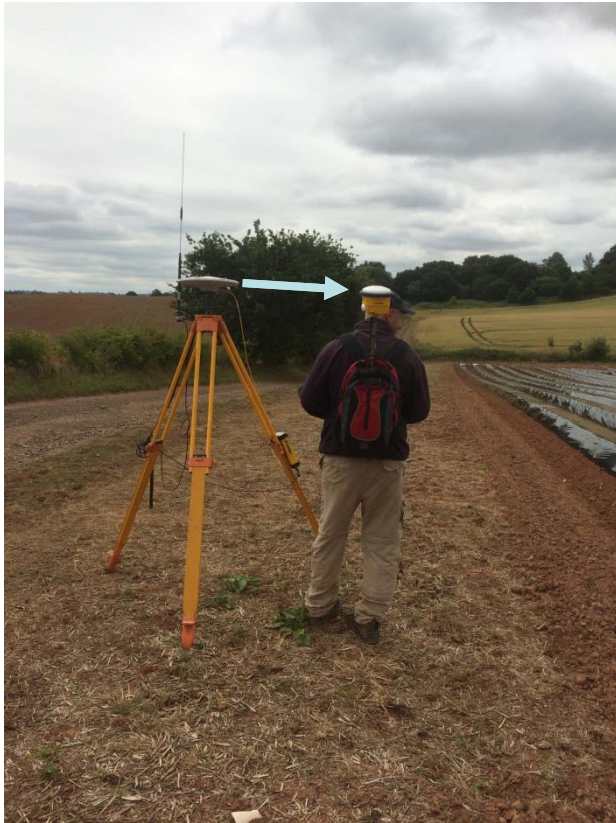
Setting up RTK Base Station
