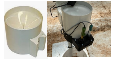
Rain Gauge with added EC/Ph Sensor well
